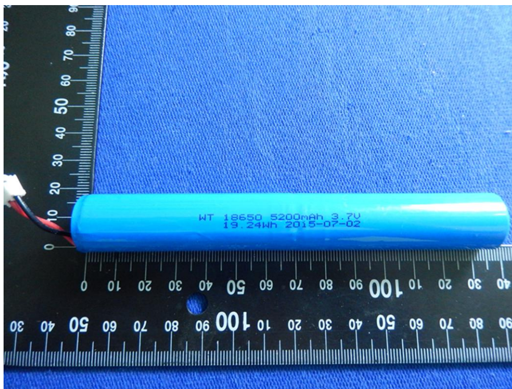
Battery (WT 18650 3,7V 5200mAh 19,24Wh)
